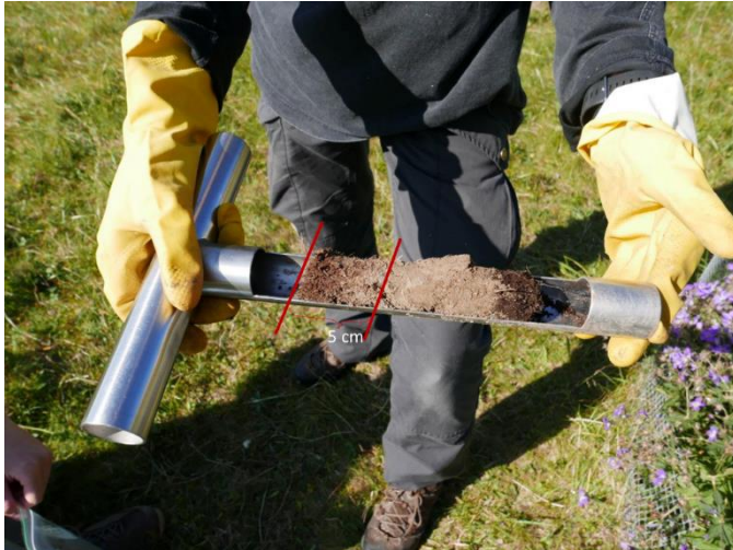
Figure 7. A soil core showing the top 0-5 cm part we collect. Here the top 5 cm includes both organic (dark) and part of mineral (light brown) horizons. This ‘soil sampling tube’ is from nhbs.com in UK.
