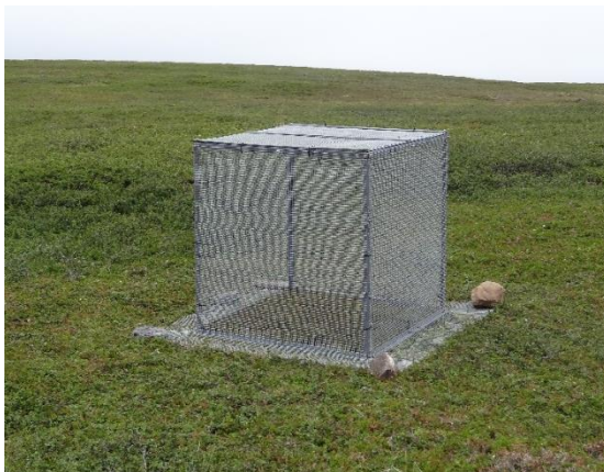
Figure 1. Experimental design within a site consists of three patches replicated within one habitat type. Each patch contains two replicates of each treatment and two control plots. This yields 8 plots per patch and 3 \times 8 = 24 plots per habitat. The large fence protects smaller cages from potential damages from for example snowmobiles or large herbivores. However, it can take any shape, or if you expect no external disturbances, you are free to build two separate large-mesh fences around the L plots.
